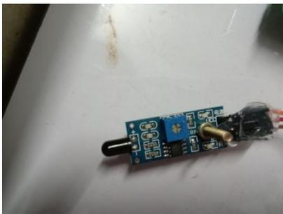
Fig .4 Diagram of Firesensor
