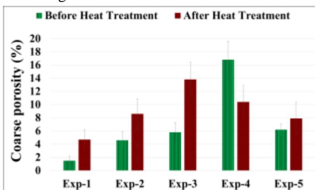
**Graph coarse porosity content in % area for all coatings before and after heat treatment**
