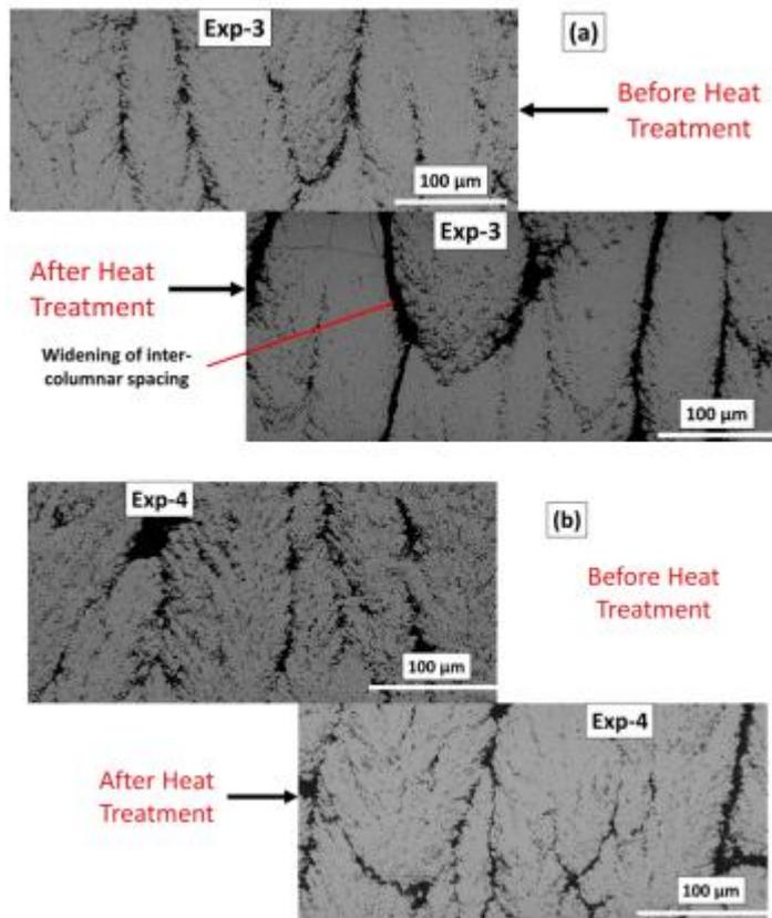
**Figure SEM micrograph of the cross-section of coating Exp-3 (a) at lower magnification showing the coarse porosity before (up) and after (down) heat treatment confirming the pore coarsening (widening of inter-columnar spacing)**
