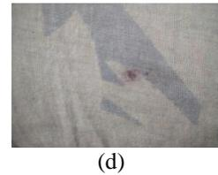
Figure 1 represents the different types of fabric defect samples (a)Hole (b)Carring (c)Knot (d)Dark spot
