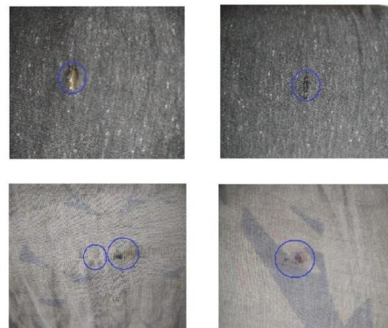
Figure 4. The fabric defect inspection results for the fabric image
