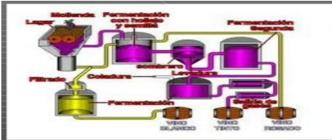
Fig 2 Block Flow diagram for wine production
