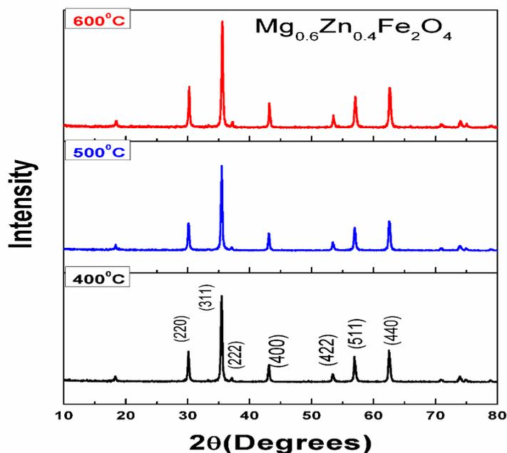
Fig(1) XRD patterns of 0.6 M % Mg-doped ZnFe<sub>2</sub>O<sub>4</sub> sample calcinated at 400°C, 500°C and 600°C
