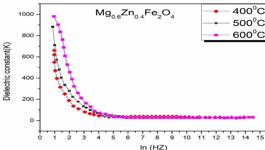
Fig(5) Variation of Dielectric constant of  $Mg_{0.6}Zn_{0.4}Fe_2O_4$  with Applied frequency
