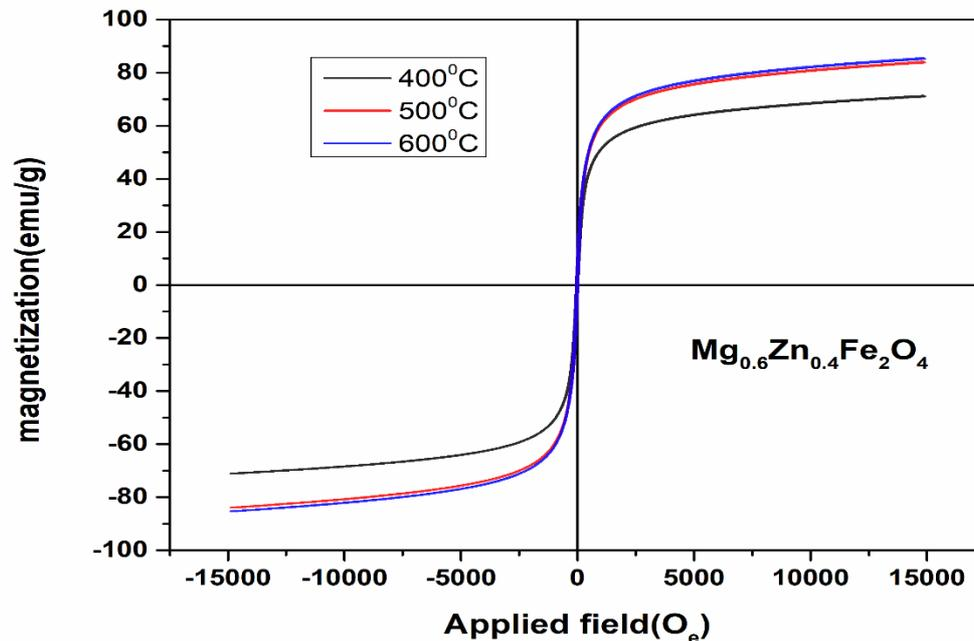
Fig(6) Variation of Saturation Magnetization of  $\text{Mg}_{0.6}\text{Zn}_{0.4}\text{Fe}_2\text{O}_4$  with Applied field at 400°C, 500°C and 600°C
