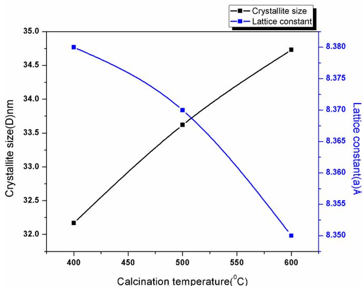
Fig(2) Variation of Crystallite size and lattice constant of Mg<sub>0.6</sub>Zn<sub>0.4</sub>Fe<sub>2</sub>O<sub>4</sub> sample at 400°C, 500°C and 600°C
