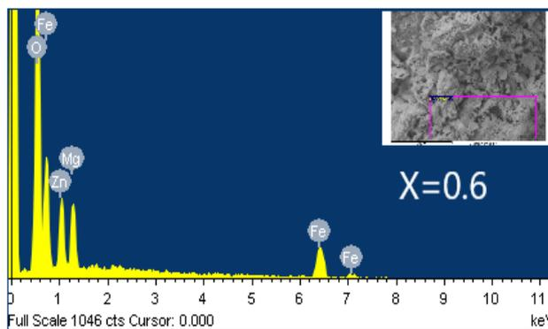
Fig(4) EDS image of  $Mg_{0.6}Zn_{0.4}Fe_2O_4$  ferrite sample
