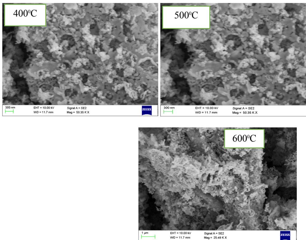
Fig(3) SEM images of  $Mg_{0.6}Zn_{0.4}Fe_2O_4$  ferrite sample at 400°C,500°C and 600°C
