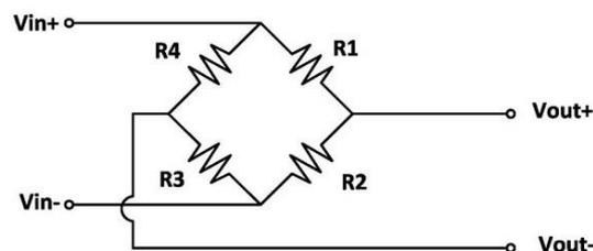
**Figure Circuit diagram of load cell sensor**
