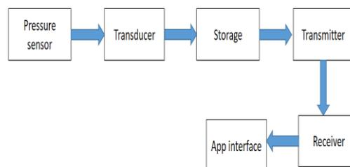
Sensors used will provide the gait analysis. The output of the sensors (piezo-electric, flexi-force, capacitive and resistive) is given as input to the transducer. The transducer produces the output in the form of voltage. This voltage is used to store the data in RAM. The RAM used is of 500 MB. Then the output is given to the transmitter. The transmitter used here is bluetooth transmitter of frequency 2.4 GHz and it covers a range of 100m. This
