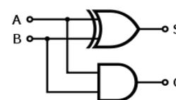
Fig 2.1: Half Adder Logic Diagram
