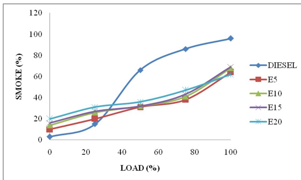
Fig. 4 Variation of Smoke emission with respect to change in load
