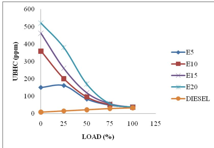
Fig. 5 Variation of hydro carbon emission with respect to change in load
