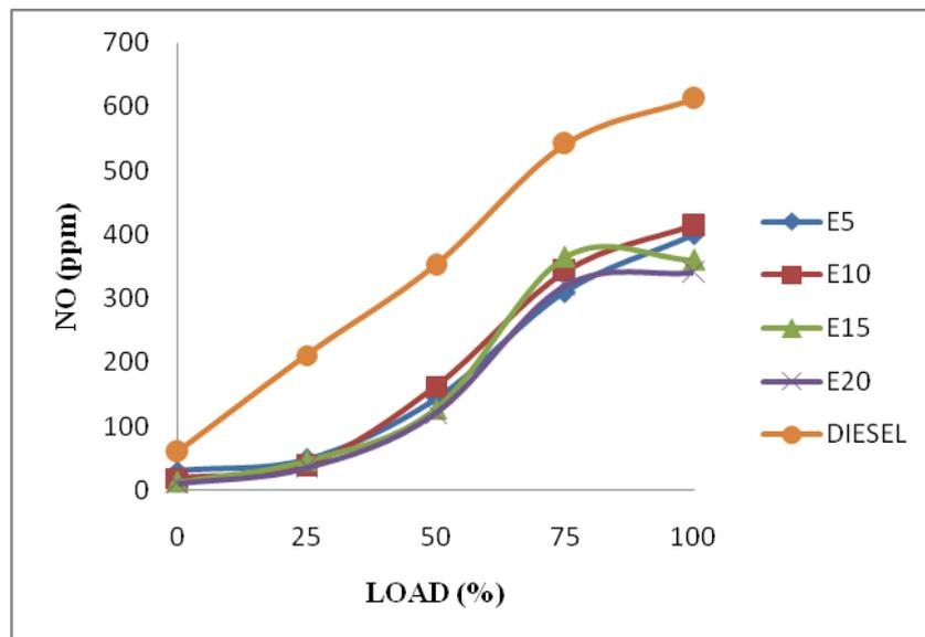
Fig. 3 Variation of NO<sub>x</sub> emission with respect to change in load
