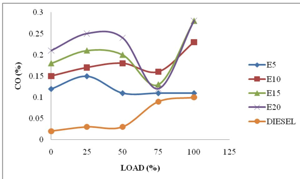
Fig. 5 Variation of carbon monoxide emission with respect to change in load
