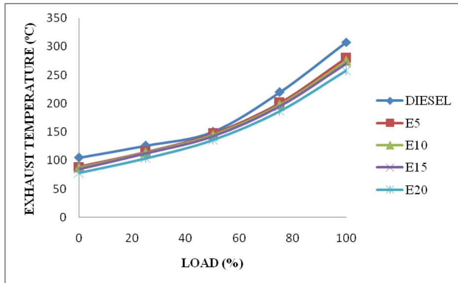
In this research work, it is noted that exhaust gas temperature was increases with increase in operating load condition and decreases with increase in ethanol blending ratio. High latent heat of vaporization of ethanol produce low temperature combustion which causes lower exhaust temperature compare to conventional diesel combustion.
