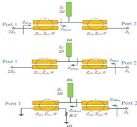
Figure 2: Equivalent circuit of the Filtering power divider [12].
