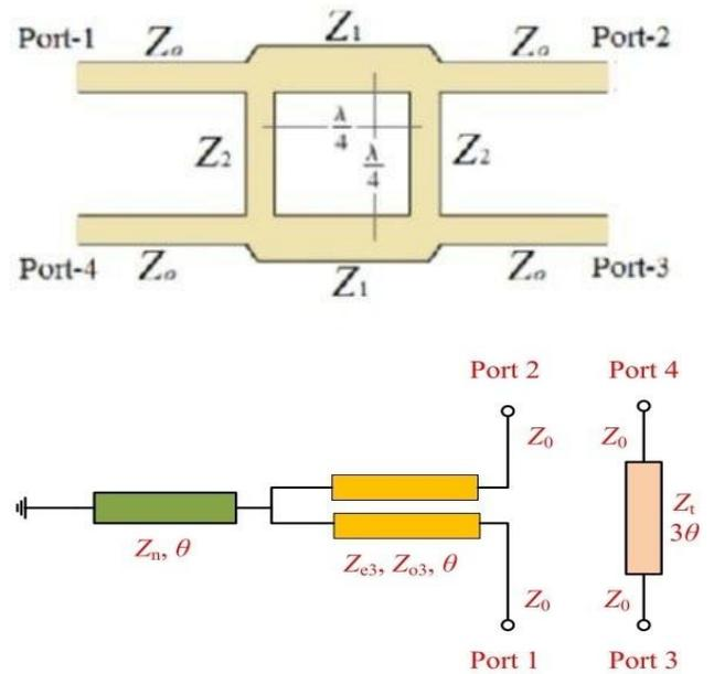
Figure 3: The circuit configuration of the Wide-band coupled-line phase shifter [13].
