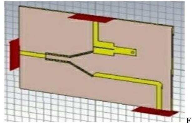
FIG 5. The circuit layout of proposed metamaterial inspired three port couplers.
