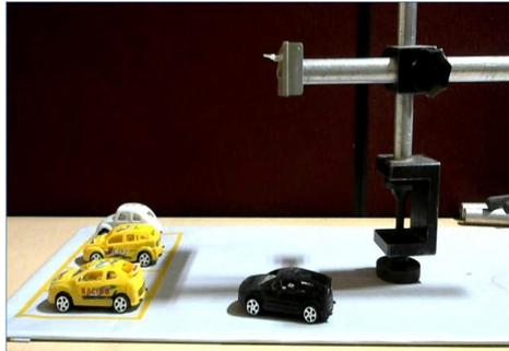
Fig. 1 Model of proposed intelligent car parking system
